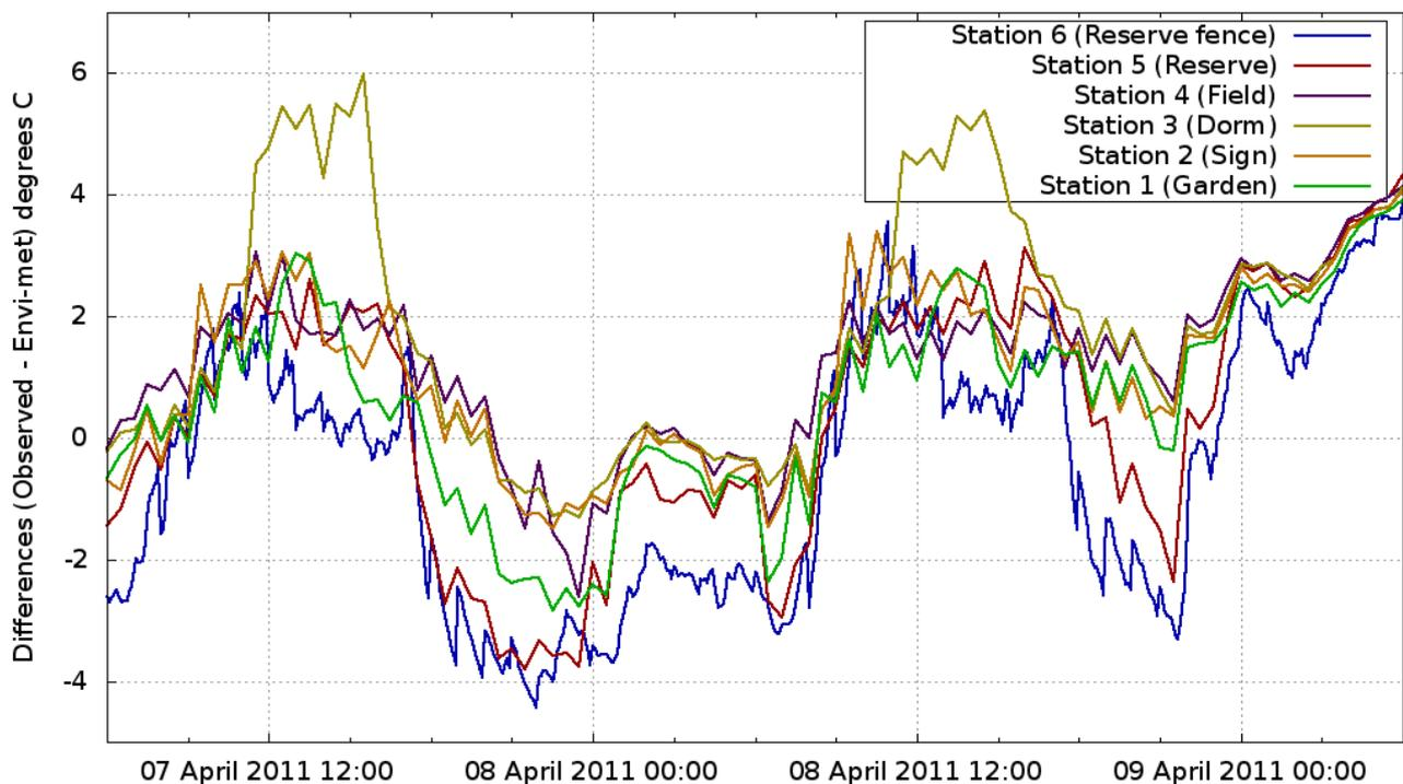
Figure 15–Differences in temperature between observation sites and ENVI-met model results, 7-8 April 2011
