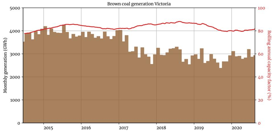
**Figure 2: Monthly output of brown coal generators in Victoria since the beginning of financial year 2014. The closure of the Hazelwood power station in early 2017 resulted in improved fleet-wide capacity factor. This fleet-wide capacity factor has since deteriorated and is expected to continue declining, as more renewable energy capacity enters the system.**
