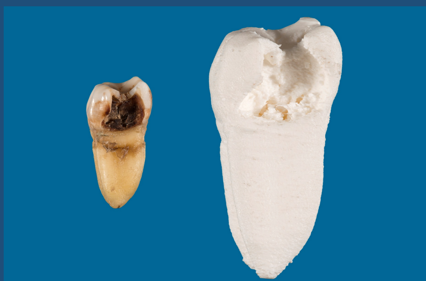
Fig. 6 Tooth specimen (left) and a 3D print of a microCT scan of the same tooth. The print was of an enlarged version of the 3D model made with the scan.
