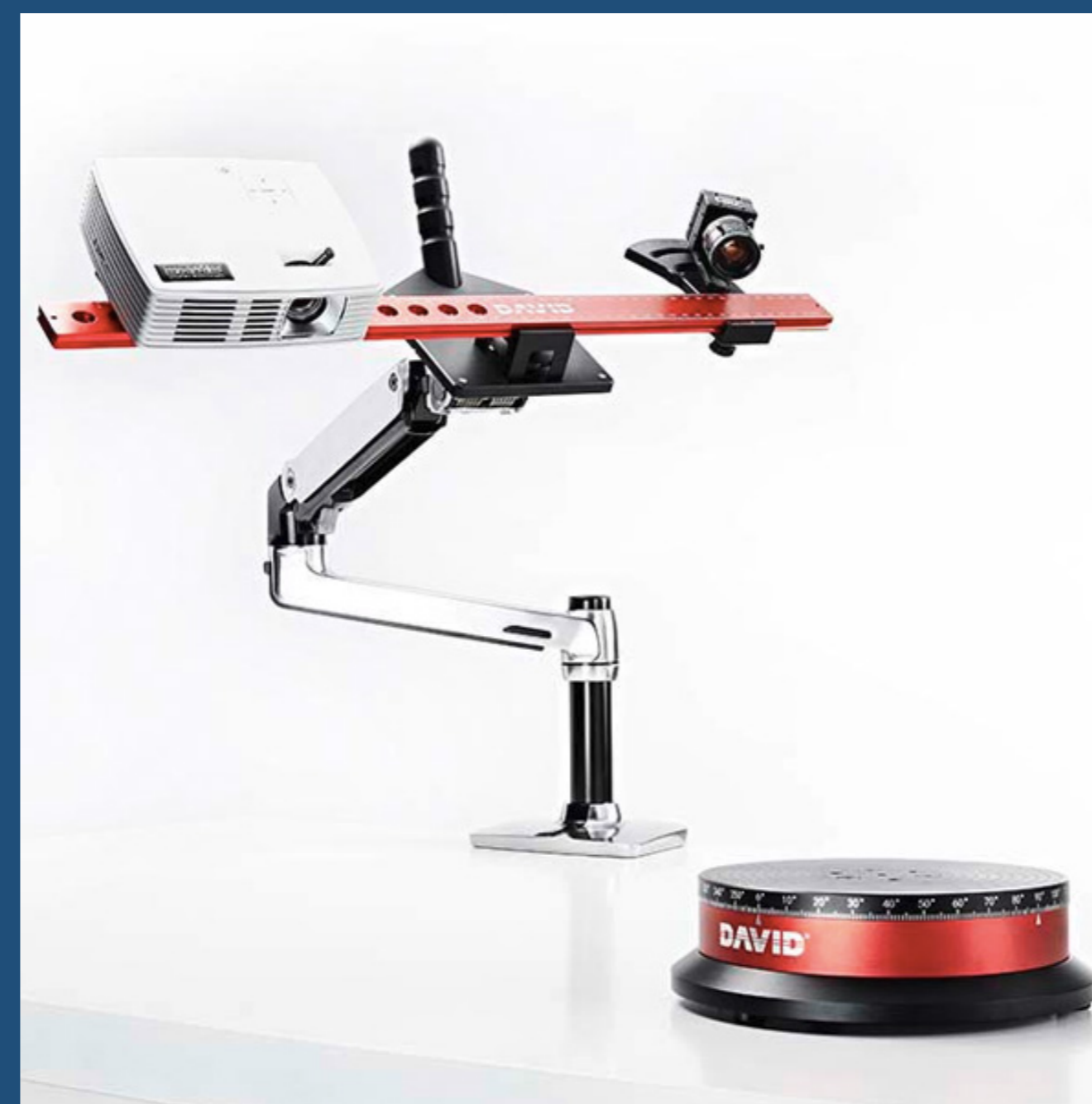
Fig. 3 DAVID SLS3 surface scanner with electronic turntable. Image source: aniwaa.com
