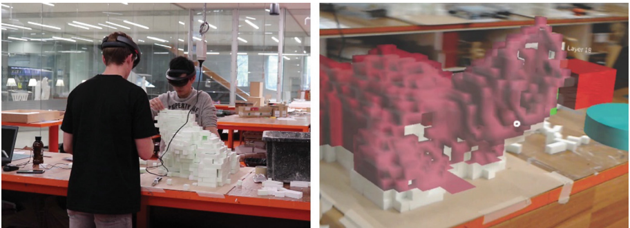
Fig. 10. Nest-scale augmented-reality assembly process. Left: Augmented reality headsets used to guide the placement of modules. Right: Point of view from headset.
